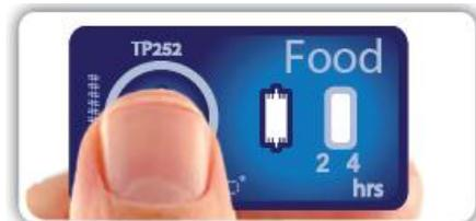
**To Activate:** Fully squeeze the button on top of the indicator. A blue line and ON will appear. Within five minutes, place the Timestrip® Food below its STOP temperature (3°C/37°F) for a minimum of two hours. The product to be monitored must also be at or below the STOP temperature when the indicator is applied to avoid a premature indication.
