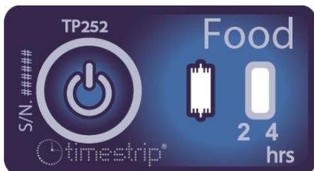
The Timestrip® Food indicator monitors time elapsed at or above 5°C/42°F for up to four hours and stops monitoring it at or below its STOP temperature (3°C/37°F). It is inert until activated and can be stored at room temperature until needed. It is self-adhesive, single use and irreversible. It has a pre-activation shelf life of two years from shipping and a one year active shelf-life.
