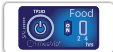
**Review:** When the threshold temperature (5°C/42°F) is breached the blue dye will move across the scale showing the cumulative time the Timestrip® Food indicator has been exposed above this threshold. The progress of the blue dye is irreversible but will stop each time the product is returned to its STOP temperature (3°C/37°F).
