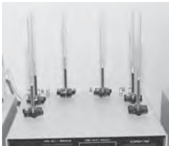
Figure 6. Dynatherm Six-Tube Conditioner with the Tubes In-Place During the Volume Challenge
