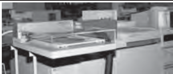
Figure 1. GERSTEL TDS A Coupled to a HP6890GC/5973MSD
